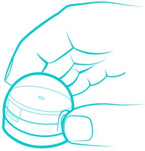
Hold down the power button on Ozobot for 2 seconds until the LED light turns white.
